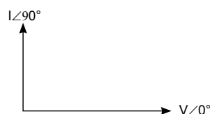
Fig. 5.17: Phasor Diagram a pure capacitive circuit
