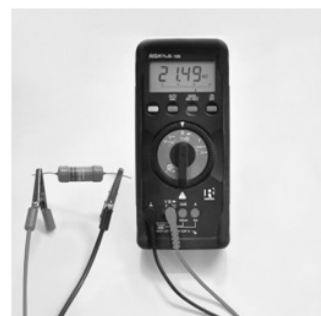
Fig. P13.2: Resistance Measurement using Digital multimeter
